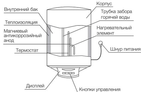
**Рис. 2. Heatronic DL DryHeat, Heatronic DL Slim DryHeat**
